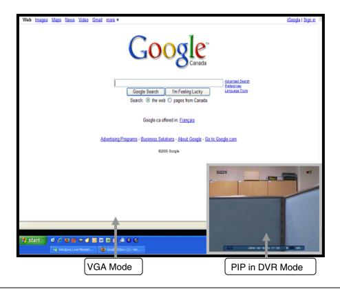
Note: When in VGA, Component, or Picture Frame Mode, the PIP window will only display DVR Mode.
